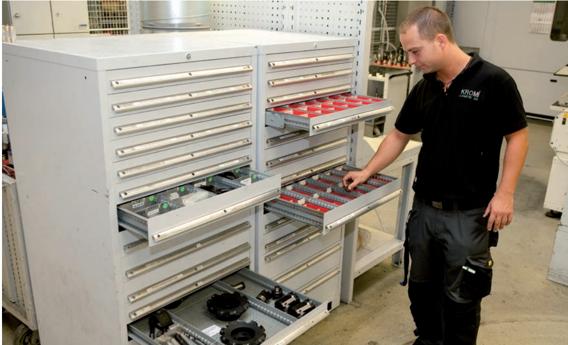
Kanban systems are perfect logistics solutions for replacement parts in production
